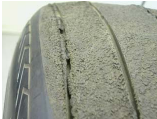
FIGURE 5: CLOSE-UP OF REVERTED RUBBER TIRE DAMAGE.
