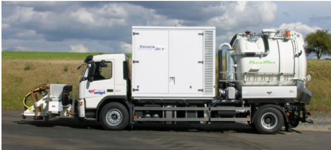
FIGURE 7: TRACKJET VEHICLES USED FOR AIRPORT RUNWAY CLEANING
