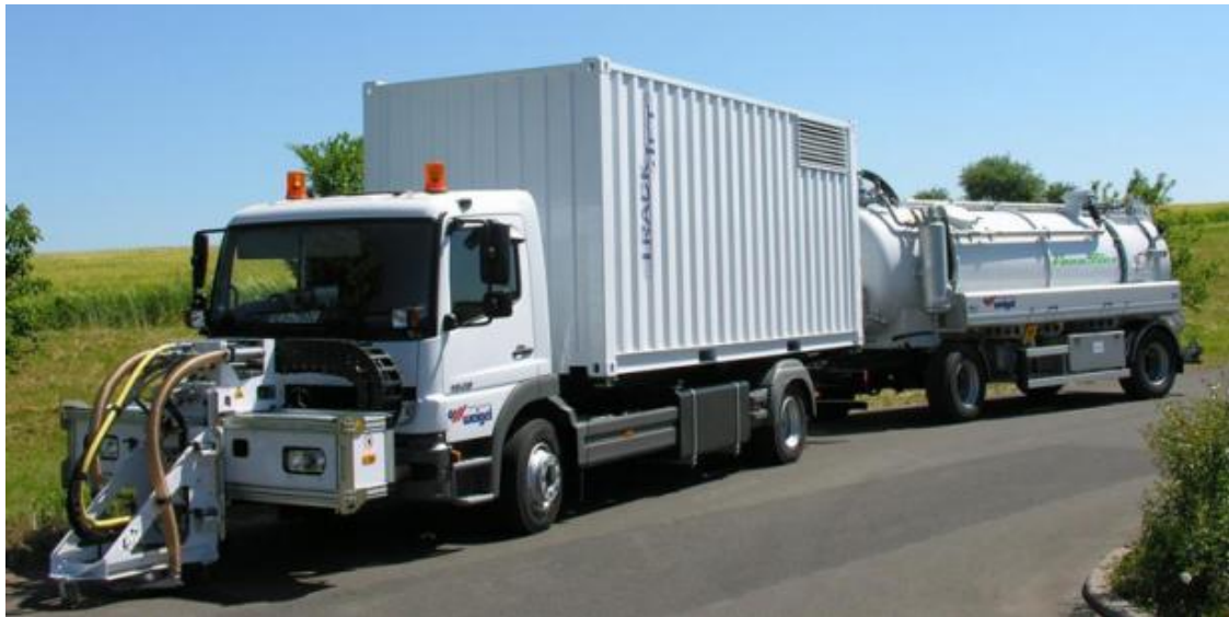
FIGURE 8: AIRPORT RUNWAY HIGH PRESSURE WASHING VEHICLES
