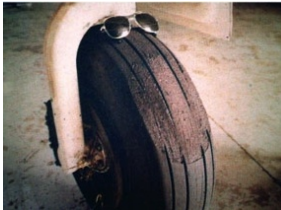
FIGURE 4: REVERTED RUBBER HYDROPLANING DAMAGED TIRE.
